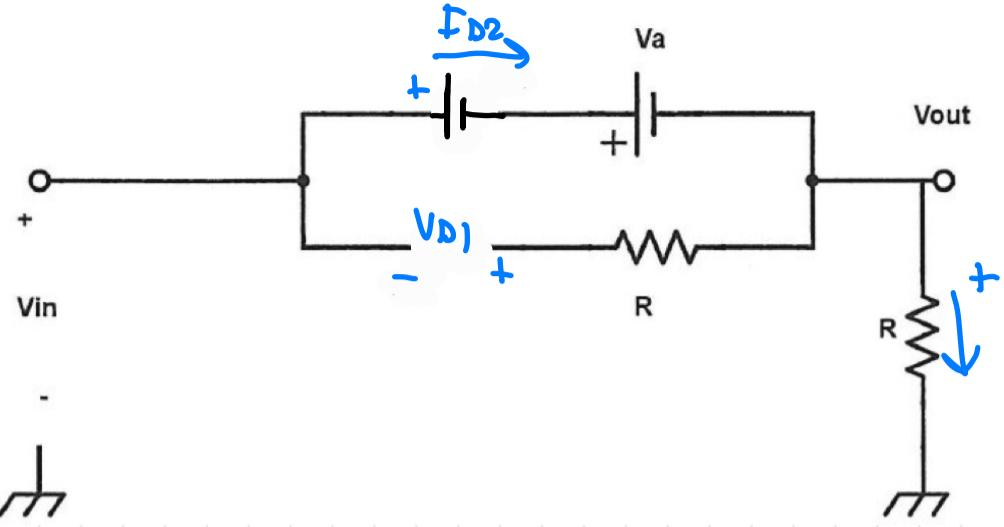
$$\bullet V_0 = R \frac{V_g - V_g - V_d}{R} = V_d - 5.7$$
