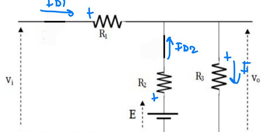
$$\left\{ \begin{array}{l} V_0 = R_3 I \\ V_0 = E - R_2 I_{D2} \\ V_0 = V_x - R_1 I_{D1} \\ I = I_{D1} + I_{D2} \end{array} \right.$$
