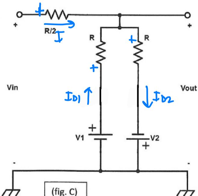
$$\bullet \begin{cases} V_O = V_1 - R I_{D1} \\ I_{D2} = I + I_{D1} \\ V_O = -V_2 + R I_{D2} \\ V_O = V_i - \frac{R}{2} I \end{cases} \rightarrow \begin{cases} V_O = V_1 - R I_{D1} \\ V_O = V_i - \frac{R}{2} I \\ V_O = -V_2 + R I + R I_{D1} \end{cases}$$
