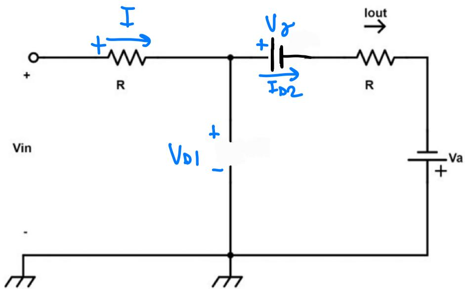
$$\bullet i_0 = I_{D2} = I = \frac{V_i - V_g + V_a}{2R} = \frac{V_i - 4}{2R}$$
