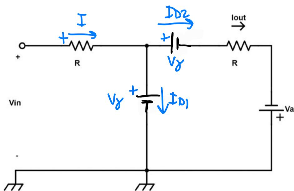
$$\bullet i_0 = I_{D2} = \frac{V_g - V_g + V_a}{R} = V_a / R$$
