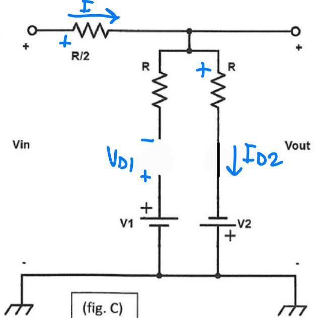
$$\bullet V_O = -V_2 + R I_{D2} = -V_2 + R \frac{V_i + V_2}{R + R/2} = \frac{2}{3} V_i - \frac{5}{3}$$
